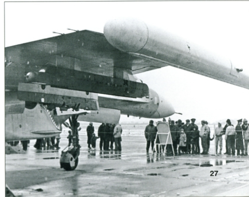
An L-005 Sorbtsiya-S (Absorption-S) jamming pod is mounted on the starboard wing tip of the Su-27 "Red 08." The covering on the front and the rear of the pod are White. A position light is mounted on the jamming pod. (Dimitry Grinyuk)
