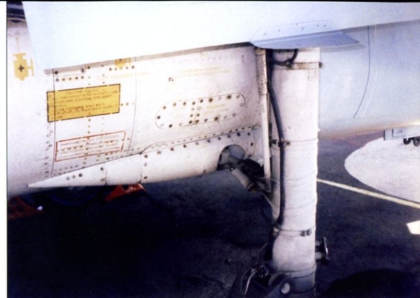
(Left) The main wheel strut of the KT-156 D main wheel, seen from the rear, has slanting main pivots. When extended, the struts are locked by mechanical down-locks mounted on the reinforced frames of the engine nacelles. (Jozef And'ál)
