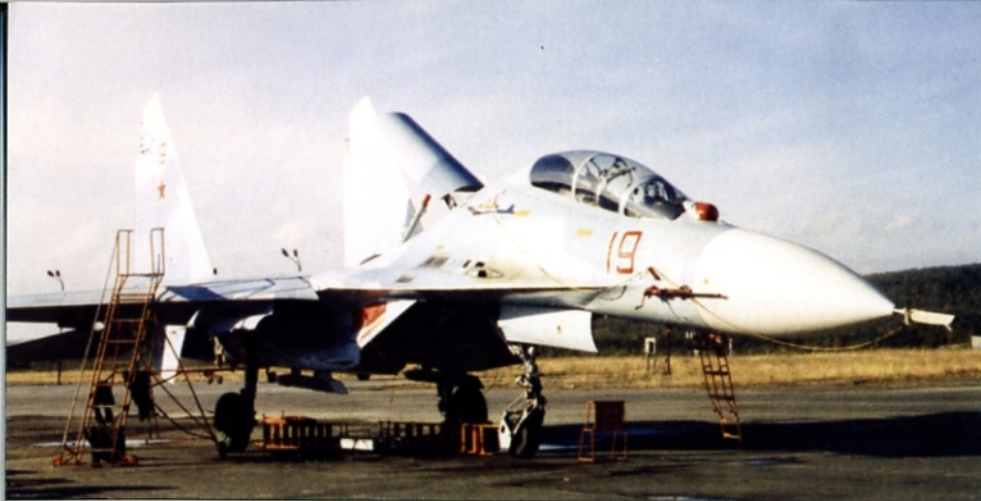
(Above) The Su-27UB "Red 19" has its air brake fully deployed. The Su-27UB had a slightly larger air brake than the single-seat Su-27 Flanker-B. A Red covering protects the centerline-mounted OLS-27 infrared search track sensor for the OEPS-27 electro-optical sighting system. The starboard bleed air spill louver on the engine nacelles is also covered. (Andrej Zinchuk)
