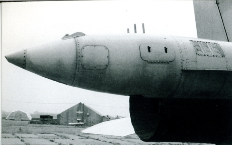
The early Su-27s have a tail sting with small lateral strakes and no box fairings. Twenty-four chaff/flare are carried by an APP-50 chaff/flare dispenser system in the early Flanker models.
