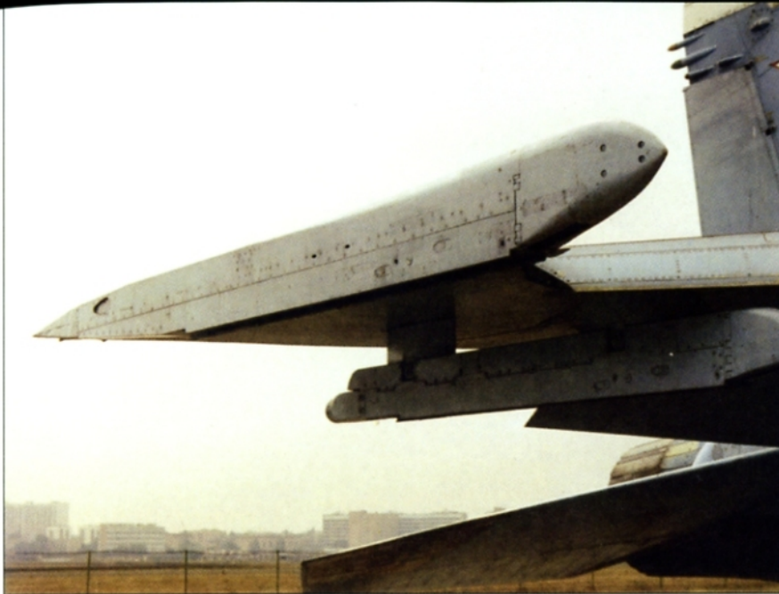
The wing tip of the Su-27 serves as a launching rail for R-73 (AA-11 "Archer") air-to-air missiles. The wing tip launching rail can be exchanged for an L-005 Sorbtsiya-S (Absorption-S) jamming pod.
