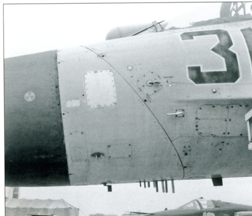
(Above left) The angle-of-attack vane is mounted on the starboard side of an Su-27 Flanker-B. The diagonal panel line divides the radome from the fuselage. The Red stenciling under the tactical number reads: "Attention! Before you lift the cone, disconnect the wave guide and cables through the hatch number 101-1AL. Before you remove the cone, lift it up. Disconnect the cable from aerial AP-038, pipes from PVD, and the connector of the PVD heating." (Pavel Türk)
