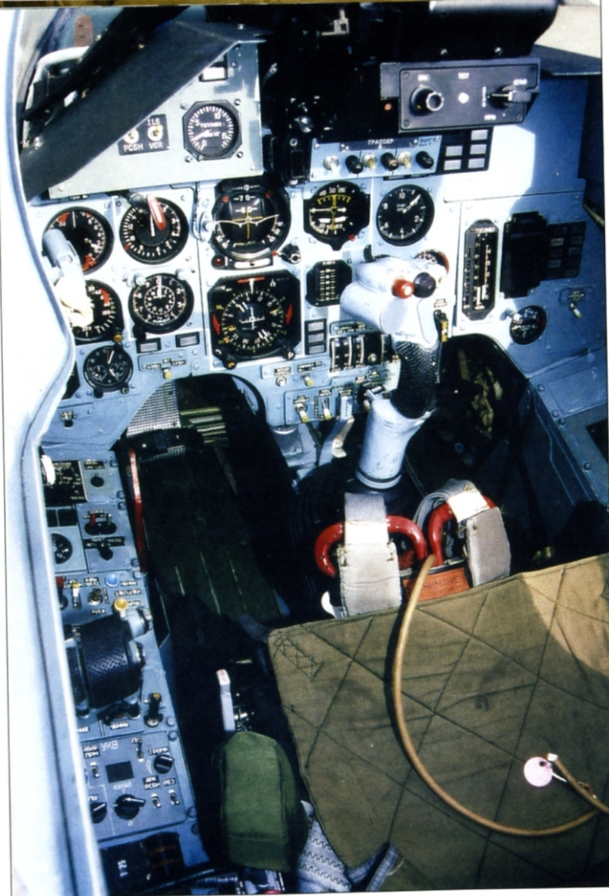
The cockpit of this Su-27 Flanker-B has been modified for air shows in Western Europe, Asia, and North America. The upper left instrument panel has been modified, and the inscription is in English. Several buttons have been removed from the control stick, and the apertures have been faired over. The radar/IRST CRT display is also missing from the upper starboard side instrument panel. Instead, the panel has been faired over. (Marcus Fülber)
