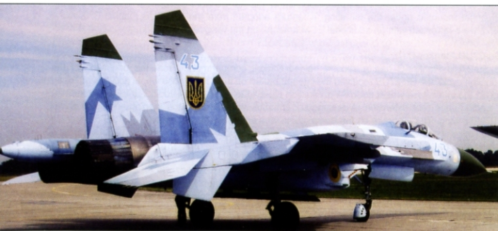
This Ukrainian Su-27 is an early-production Flanker-B. The early Su-27 has a tail sting with small lateral strakes and no box fairings. The early models of the Flanker carried 24 chaff/flare dispensers. Early Su-27s had a mudguard with three apertures on each side on the KN-27 nose wheel as well as a Green radome. The splinter camouflage is typical of Flankers belonging to the Ukrainian Air Force. (Marcus Fülber)
