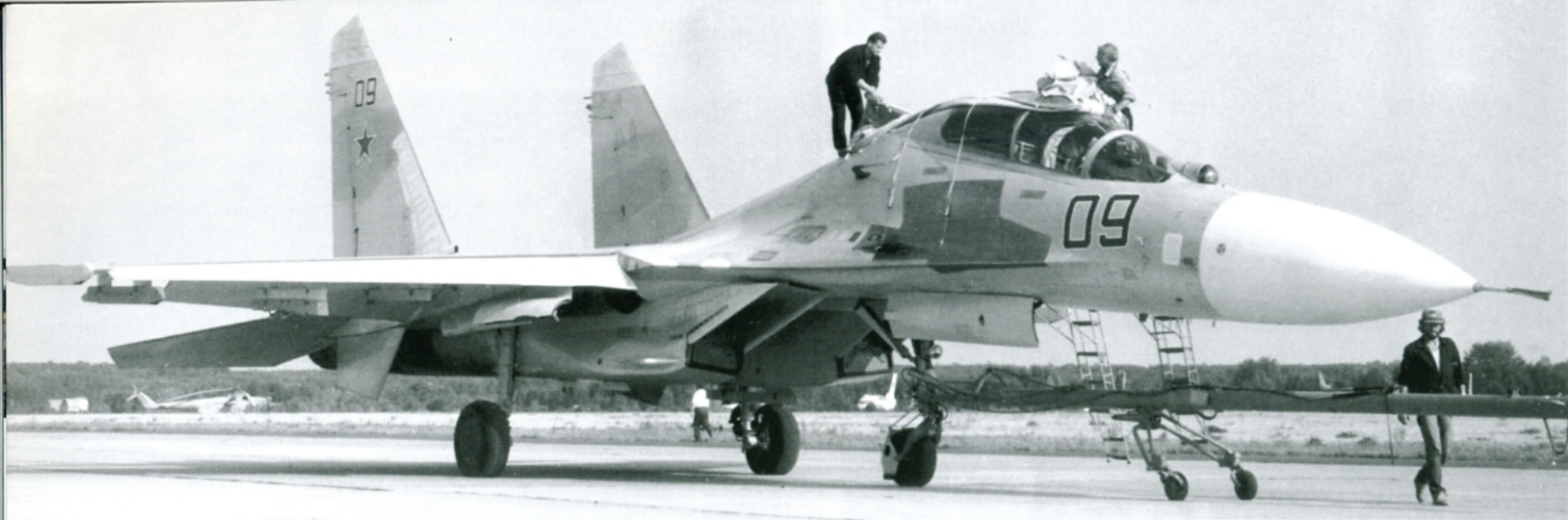
This Su-27UB "Blue 09" clearly shows the antenna configuration of the Flanker trainer. Two ECM antennas are mounted on the leading wing edge. These are usually painted White, but some Su-27UBs have them painted Radome Green. Another antenna is located on the wing leading edge
