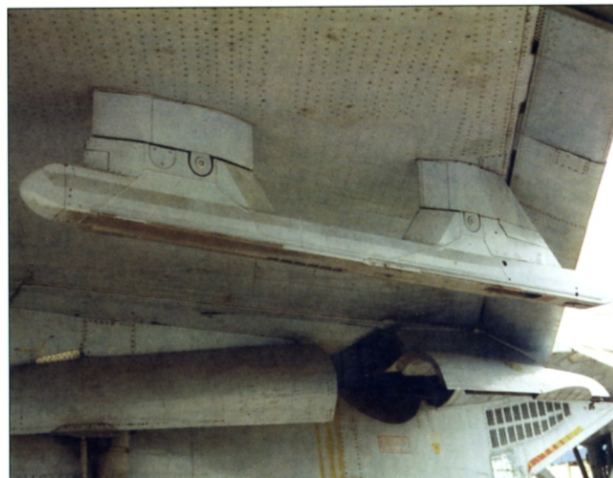
The inner APU-470 wing pylon carries R-27 (AA-10 "Alamo") air-to-air missiles.
