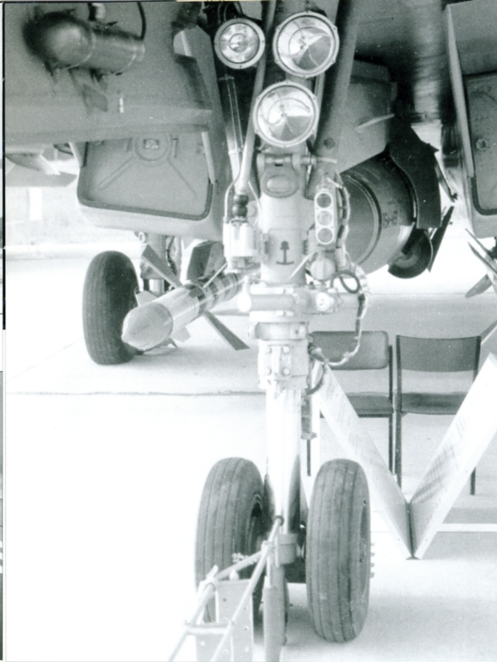
The Su-27K has a twin nose wheel with a reinforced nose wheel strut. The position of the landing and taxiing lights differs from those on the Flanker-B. A three-color light indicator on the port strut informs the flight controller on deck about the Flanker's position on the glide path and its landing speed.
