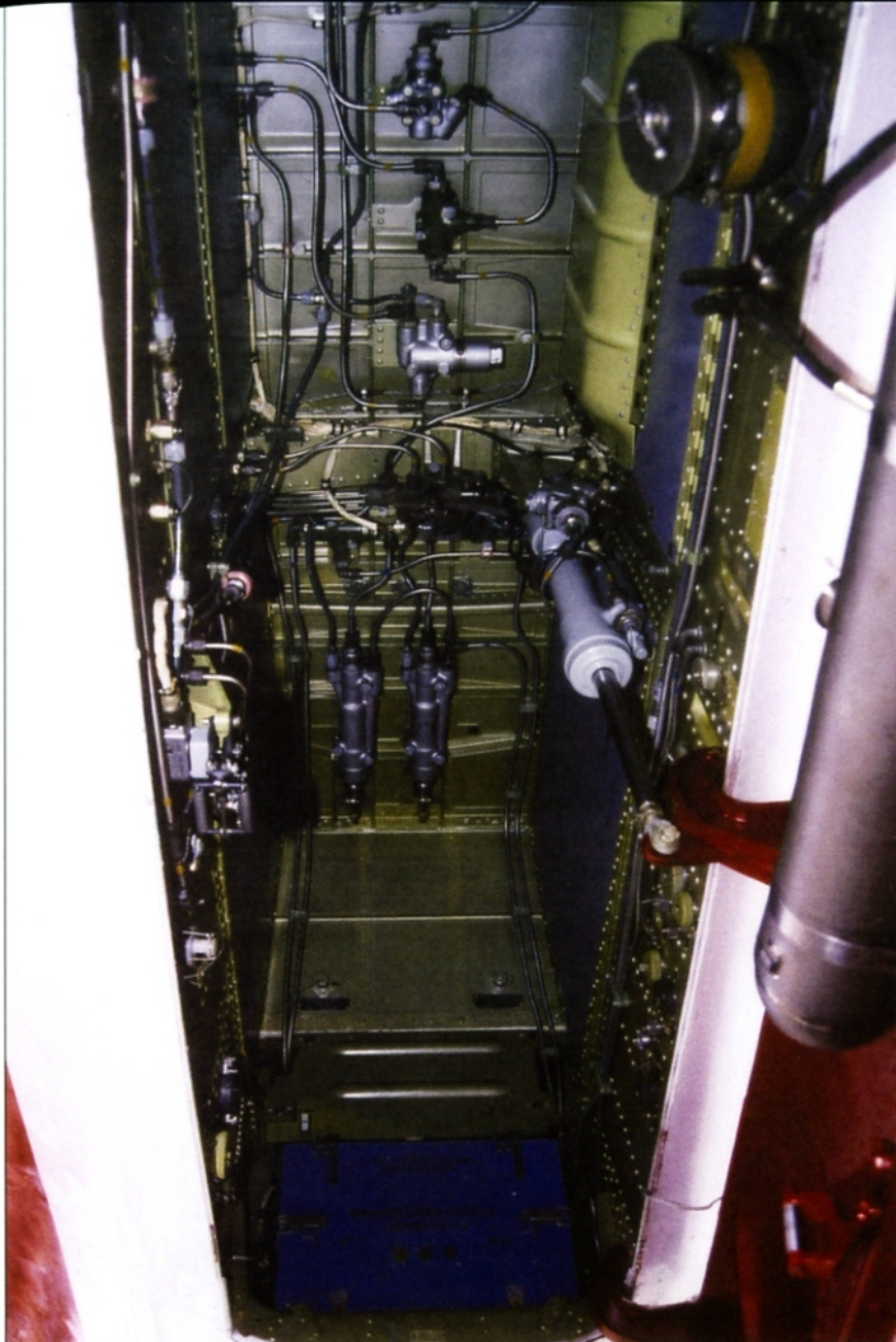
The central refueling point is located above the glycol tank in the nose wheel well of a late-production Su-27 Flanker-B. It was introduced in late-production Su-27s, making refueling the plane much easier. On earlier models, the ground crew had to climb to the dorsal spine to access refuel points. (Marcus Fülber)
