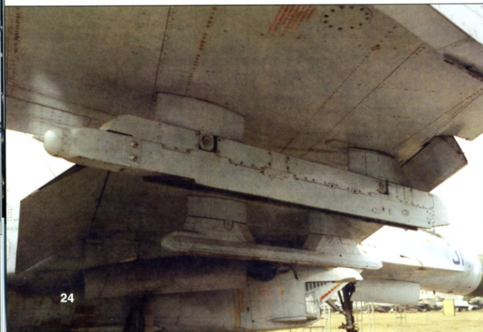
The outer APU-73 missile rail on an Su-27 Flanker-B carries R-73 (AA-11 "Archer") air-to-air missiles.
