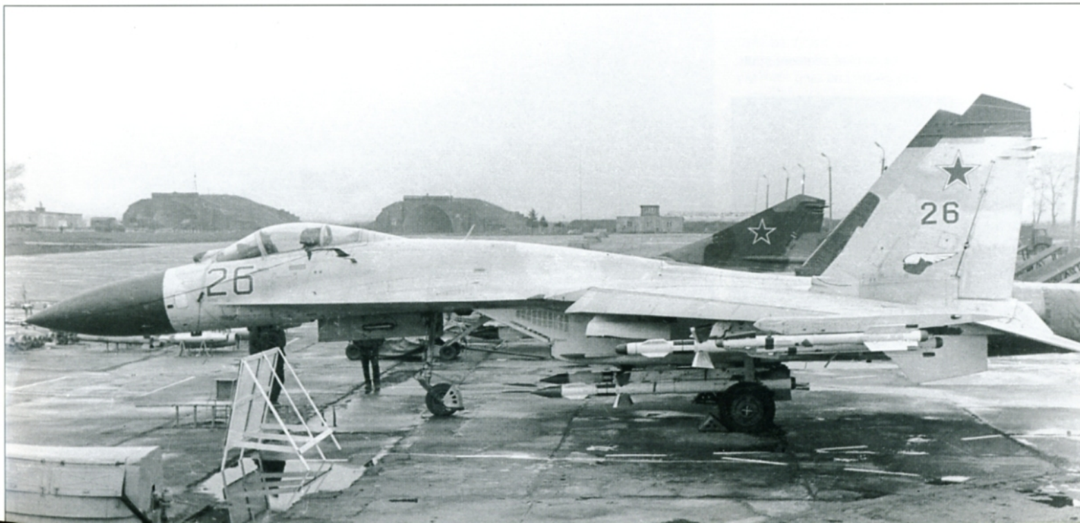
The starboard main wheel door of the Su-27 Flanker-B is hydraulically actuated. Most Su-27s have the inner surfaces of the main wheel door painted Red. However, the early-production Su-27s have the inner main wheel doors painted Gray. (Pavel Türk)
