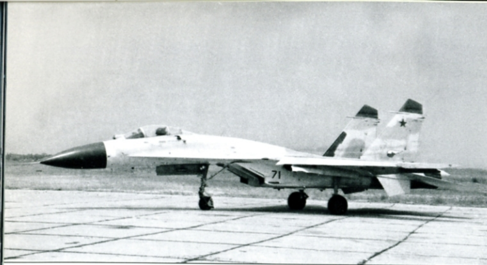
This early-production Su-27 Flanker-B fighter has anti-flutter weights on the tail fin. These weights were omitted from main-production Flankers. The inner nose wheel door lacks the bulge that is seen on standard-production Su-27s. The inside of the doors are Gray on this Su-27, "Red 71." Standard-production Flanker-Bs had the inside of the nose wheel door painted Red. ( Sukhoi OKB )
