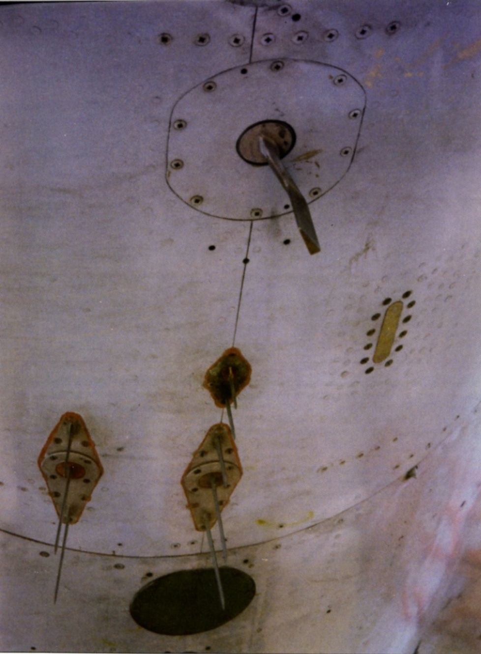
The lower nose section of an Su-27 Flanker-B is equipped with two three-pole identification friend or foe (IFF) antennas. One of the antennas is offset to the starboard side. An angle-of-attack vane is mounted in front of the IFF antennas. ( Pavel Türk )
