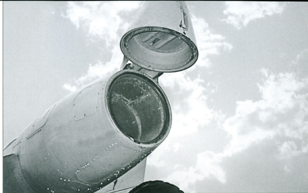
(Left) The tail sting of an early-production Su-27 Flanker-B lacks a UHF aerial. The covering for the ECM antenna is painted Radome Green, which is a typical feature for early Su-27s. The rear part of the tail sting houses two drag chutes that were covered by a conical fairing parachute door. (Urs Harnisch)
