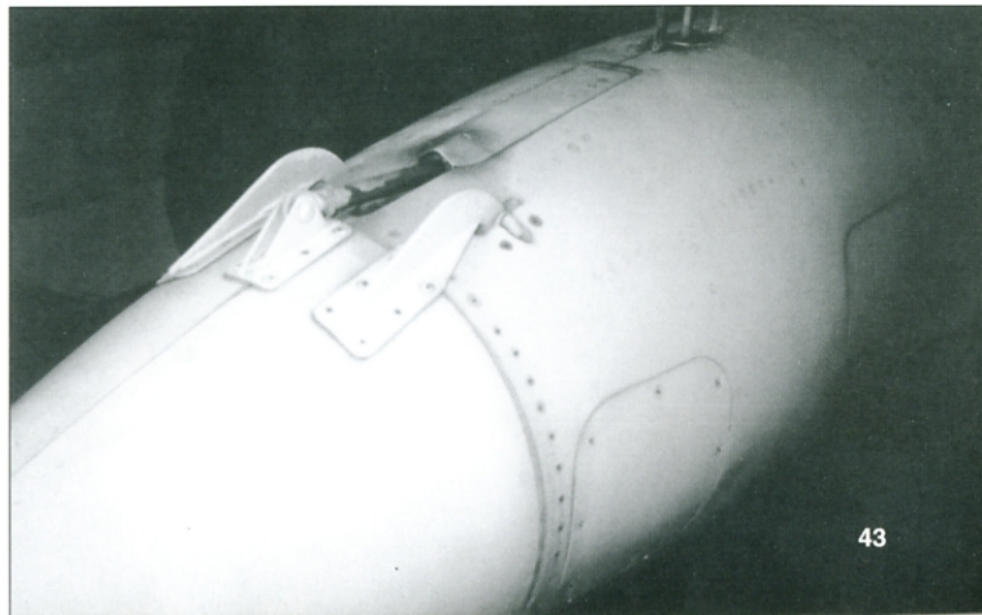
(Below) The upper conical parachute door of an early Su-27 Flanker-B has two hinges attached to the upper side of the parachute container. (Sergej F. Sergejev)
