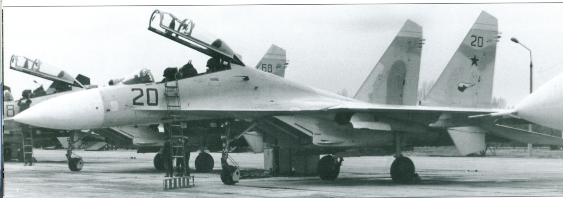
The Su-27UB "Blue 20" is a standard production Flanker-C. All production trainers are equipped with an OLS-27 infrared search track sensor mounted centerline in front of the canopy frame. In contrast to the T-10 UB-1 trainer prototype that lacked a mudguard, all Su-27UBs are equipped with
