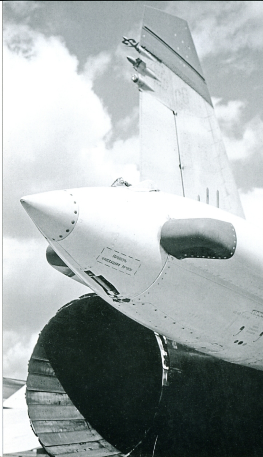
(Left) The tail sting of an early-production Su-27 Flanker-B lacks a UHF aerial. The covering for the ECM antenna is painted Radome Green, which is a typical feature for early Su-27s. The rear part of the tail sting houses two drag chutes that were covered by a conical fairing parachute door. (Urs Harnisch)
