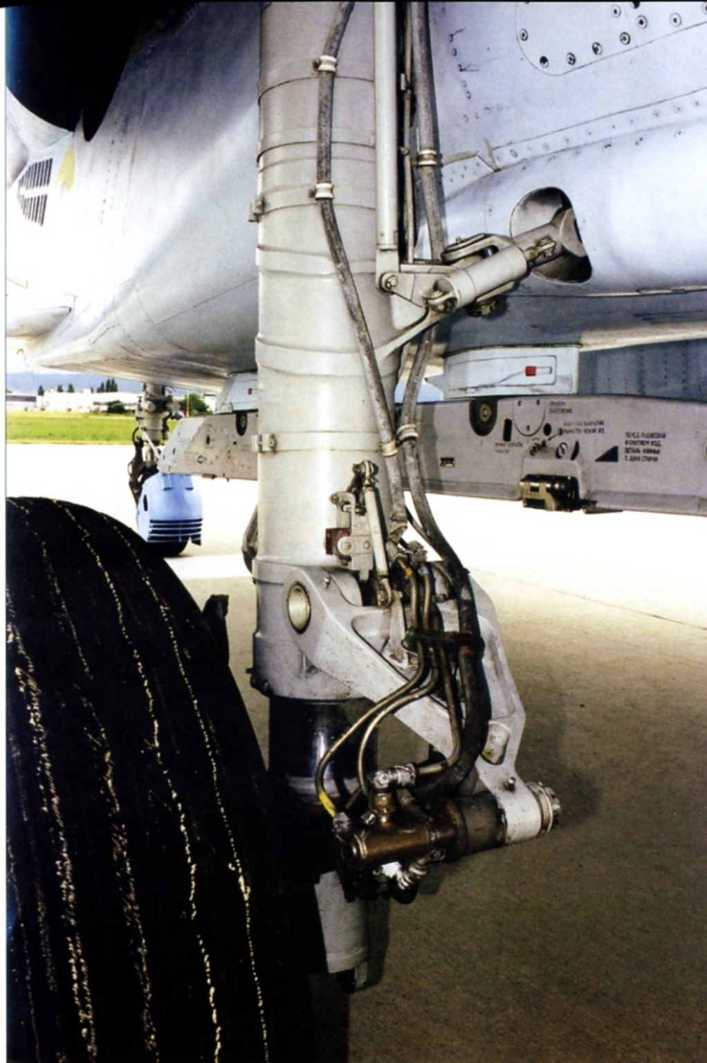
(Left) The main wheel strut of the KT-156 D main wheel, seen from the rear, has slanting main pivots. When extended, the struts are locked by mechanical down-locks mounted on the reinforced frames of the engine nacelles. (Jozef And'ál)
