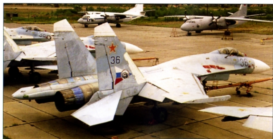
This Su-27 "Blue 36" is a late-production Flanker-B. Its revised tail sting has box fairings housing ECM antennas and 54 chaff/flare dispensers. This modification was introduced in mid-1987. Early Flankers carried 24 chaff/flare dispensers. Late-production Su-27s have the radome painted White. "Blue 36" belongs to the 941 Istrebitel'nyi Aviapolk (941st Fighter Aviation Regiment). The unit badge is painted on the starboard tail fin, and the Sukhoi logo is on the port tail fin. (Andrey Zinchuk)
