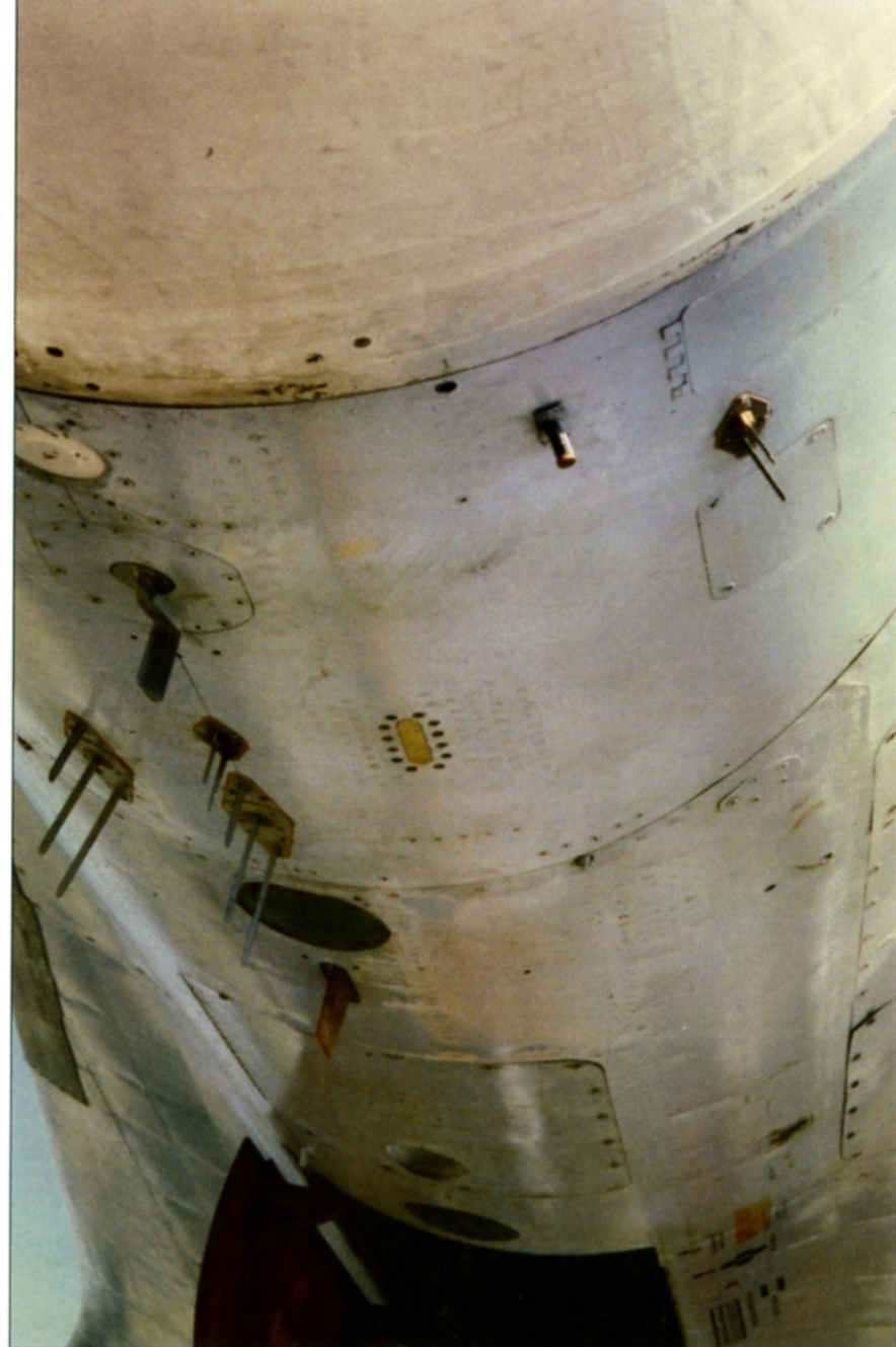
An angle-of-attack vane and two three-pole IFF antennas are visible on the lower nose of an Su-27 Flanker-B. The two two-pole antennas are also connected to the IFF system. The tube nearest the White radome is not standard for Su-27 Flanker-Bs. ( Pavel Türk )
