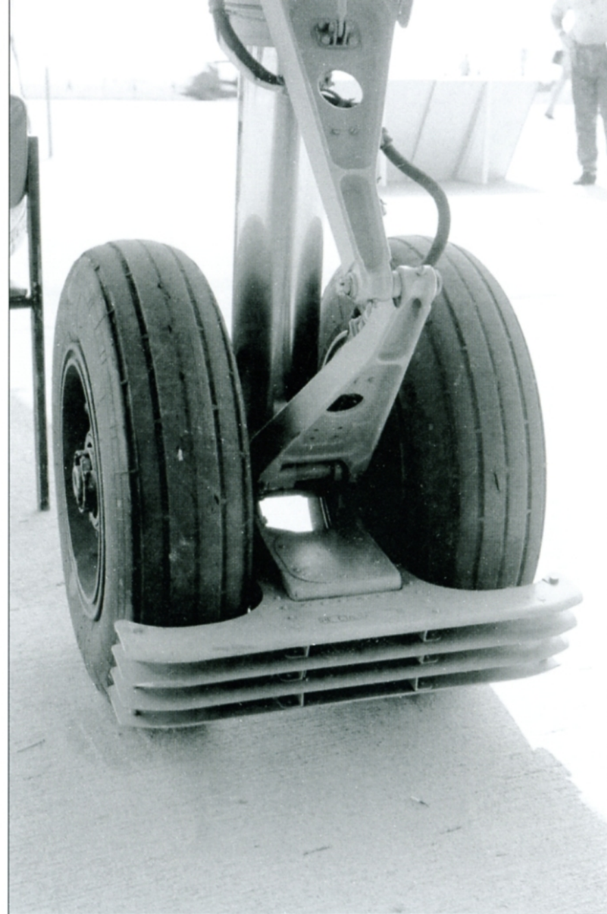
The Su-27K has a much smaller mudguard than the Su-27 Flanker-B, with no covering above the nose wheel. The twin wheels are smaller in diameter than the single nose wheel of Flanker-Bs and Flanker-Cs.
