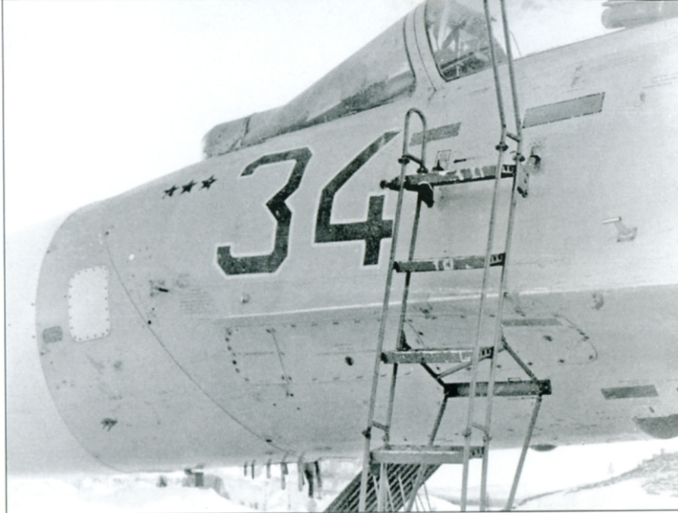
(Above left) The angle-of-attack vane is mounted on the starboard side of an Su-27 Flanker-B. The diagonal panel line divides the radome from the fuselage. The Red stenciling under the tactical number reads: "Attention! Before you lift the cone, disconnect the wave guide and cables through the hatch number 101-1AL. Before you remove the cone, lift it up. Disconnect the cable from aerial AP-038, pipes from PVD, and the connector of the PVD heating." (Pavel Türk)
