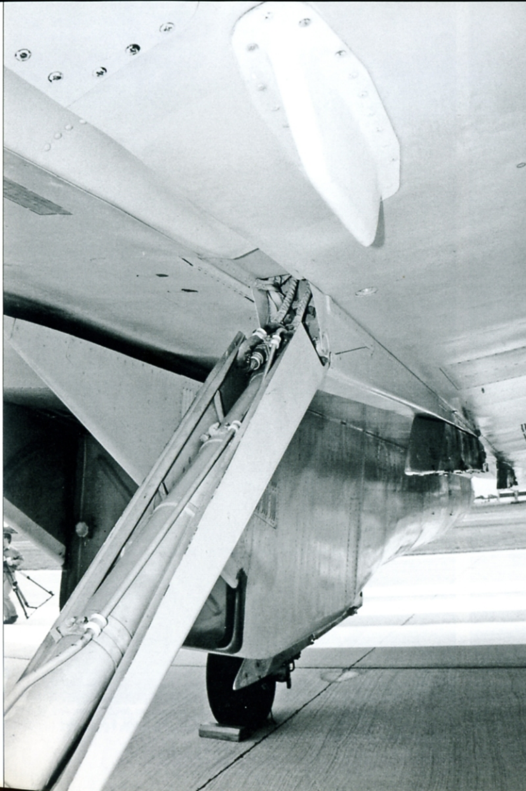
(Left) The hydraulic retraction jack of the KN-27 nose wheel has a rugged strut designed to allow the Su-27 Flanker-B to operate on unprepared fields. (Jozef And'el)
