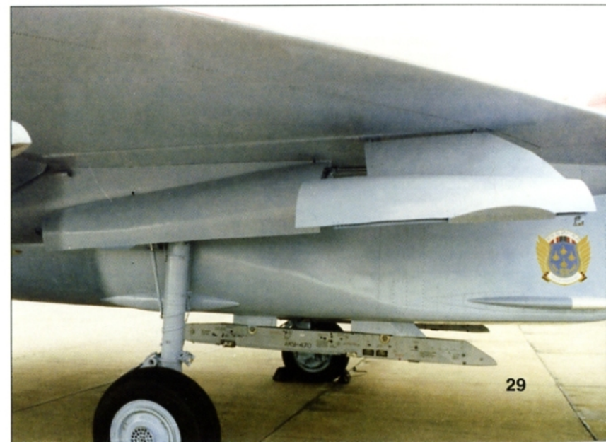
(Below) Two main wheel doors covered the KT-156 D main wheel well. The doors were hydraulically actuated. The KT-156 D retracts forward into the aft cockpit bay. (Simon Watson)
