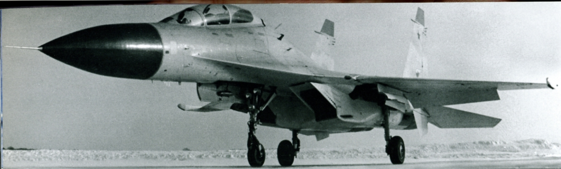
The first Su-27 trainer prototype T-10 UB-1 is shown in its original configuration. At the beginning of the flight test envelope, the first Su-27 trainer lacked the OLS-27 infrared search track sensor mounted centerline in front of the canopy frame. The T-10 UB-1 adopted the horizontal tail
