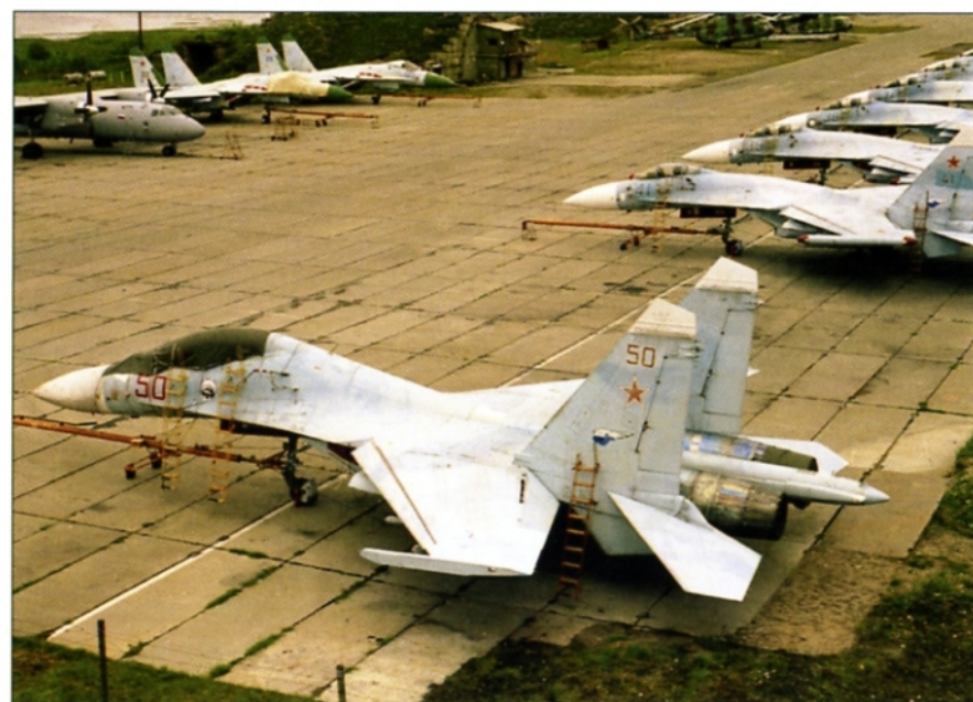
The Su-27UB Flanker-C "Red 50" shares Kilp-Yavr airfield in Murmansk with single-seat Su-27 Flanker-B fighters. The tactical numbers being above the national marking on the tail fin is typical for Flanker trainers. The two Su-27s at the top left are early-production Flankers, as the Green radomes and tail fins denote. Standard production Su-27s have White radomes and tail fins. (Andrej Zinchuk)
