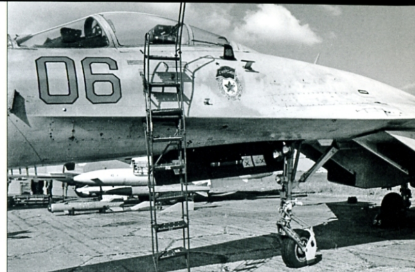
(Left) The hydraulic retraction jack of the KN-27 nose wheel has a rugged strut designed to allow the Su-27 Flanker-B to operate on unprepared fields. (Jozef And'el)
