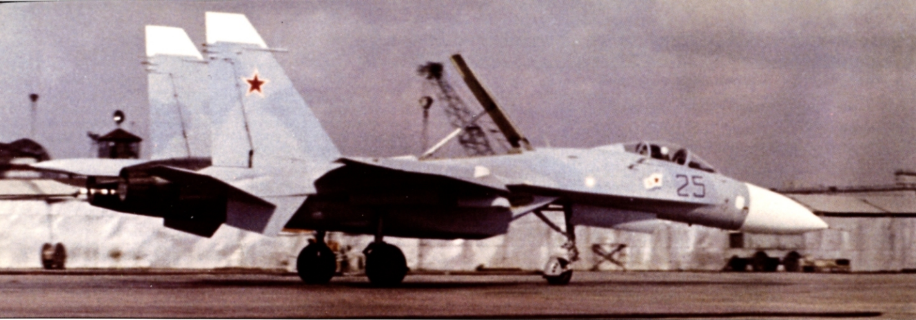
The early-production Su-27 Flanker-Bs were equipped with anti-flutter weights on the tail fins. The very early Su-27s lacked the cropped angled fin tips that became standard on production Flankers. T-10-25 "Blue 25" was one of the first series production Su-27 Flanker-Bs. This plane was manufactured at State Aircraft Factory 126 "Yuri Gagarin" at Komsomolsk-on-Amur in 1982. The T-10-25 received a retractable arrestor hook and a reinforced undercarriage in 1984. With its modifications, the T-10-25 was used as a test bed for carrier operations. Between August and October 1984, the T-10-25 performed nine arresting-gear landings. The plane was lost on 11 November 1984 because of a failure in the rudder control hydraulic system. (Sukhoi OKB)
