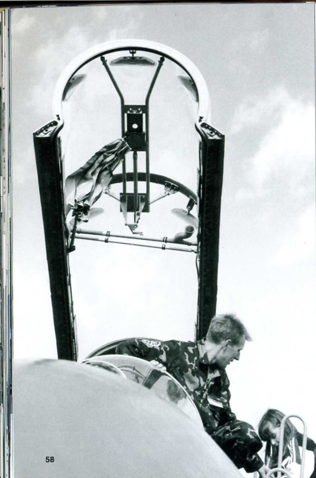
(Left) The stretched canopy of an Su-27UB Flanker-C has a suspender for a curtain in the student's compartment. Three additional rear-view mirrors are attached to the rear canopy frame. All single-seat Flanker-Bs lacked the additional mirrors and the suspender for the curtain. (Jozef And'a)
