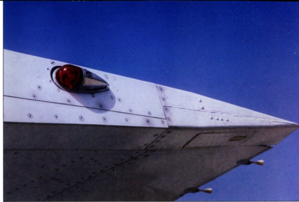
A Red position light is fixed on the port wing tip of an Su-27. Two static dischargers are located on the edge of the wing. ( Pavel Türk )
