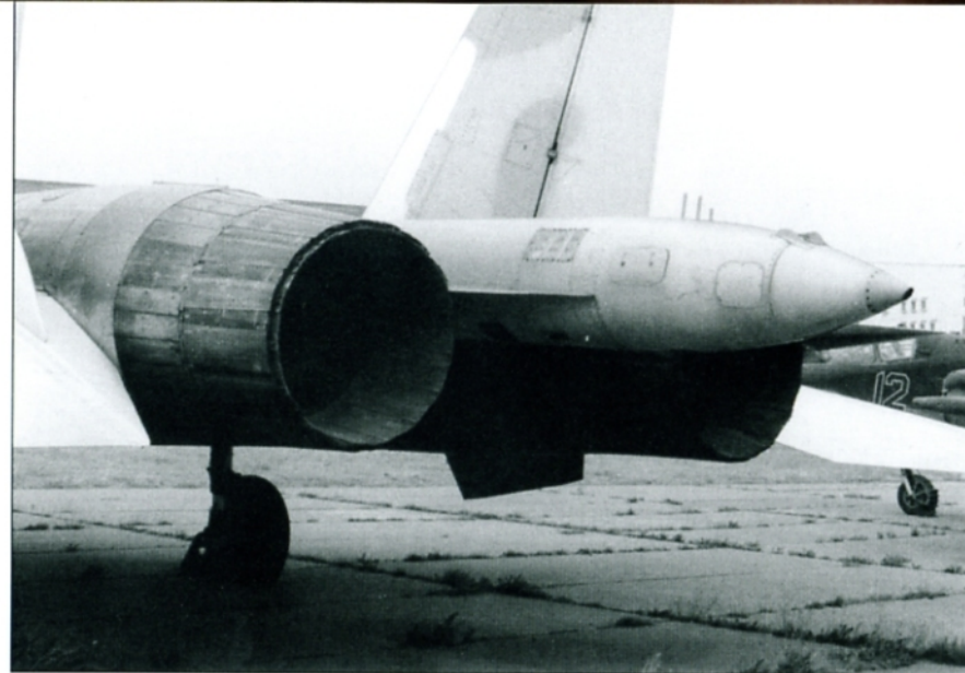
The port tail of the early-production Su-27 "Blue 31" has access hatches that were relocated on subsequent models with a revised tail sting.
