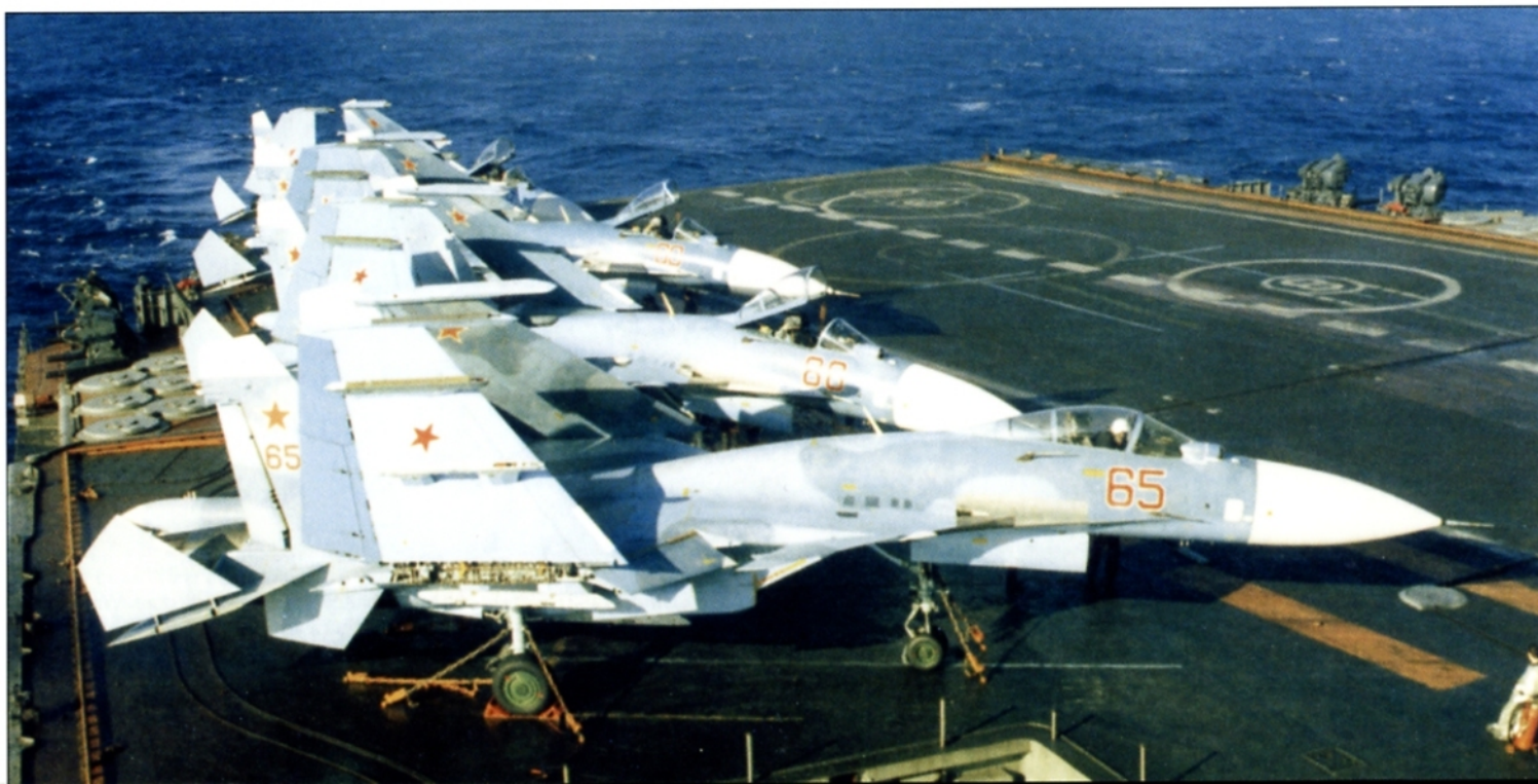
The Su-33 "Red 83" of the 279th KIAP (279 Korabel'ny Istrebitel'nyi Aviapolk/279th Shipboard Fighter Aviation Regiment) rides the elevator of the Kuznetsov from the lower hangar to the flight deck. The Su-33 had foldable wings and an all-moving tailplane. (G.F. Petrov)
